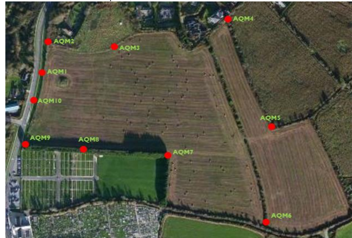
Figure 9.1 Baseline Air Quality Monitoring Locations AQM1 TO AQM10 Dust Levels Tested with DustTrak II Aerosol Monitor 8530.
