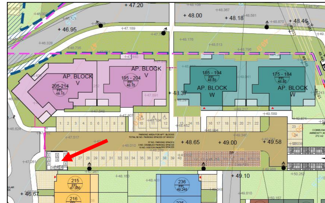
Figure 4.0 This waste storage area covers Block V & Block W (185 – 194) & Block W (175 – 184) The proposed number of bins required for this WSA including Block X, Block W (322 – 331), Block W (332 – 341) & Block W (342 – 351) is 6No. (1100L split equally for DMR and MNR) and 5 no. (240L).
